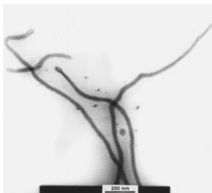
Fig. 3. Transmission electron micrograph of \gamma -Fe 2 O 3 -impregnated PBMA- b -PCEMA nanotubes with PAA-lined inner walls (reprinted with permission from Yian et al. [28], copyright 2001 American Chemical Society).
